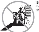
Be aware of crushing hazards when grasping the platform guard rail.
