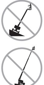
Do not raise or extend the boom unless the machine is on a firm, level surface.
