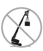
Do not place or attach fixed or overhanging loads to any part of this machine.
